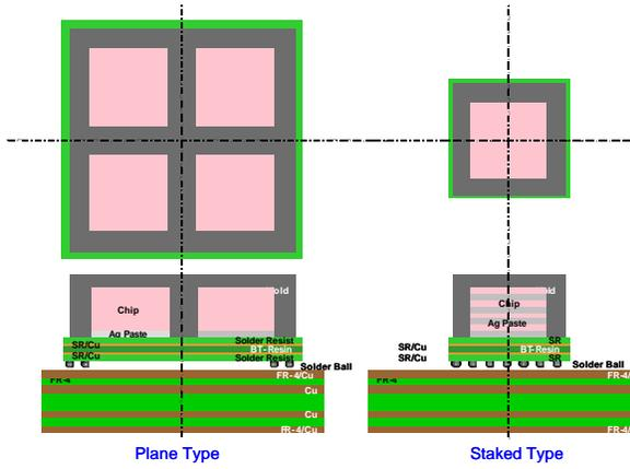
Figure 1. FEM Simulation Models for Stacked and Plane BGA
