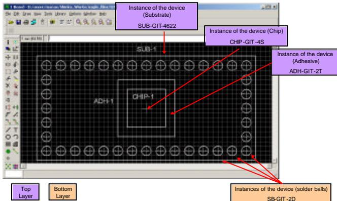
Figure 18. Chip package test case (in the EAGLE ECAD tool)
