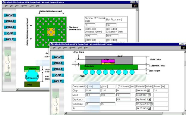
Figure 11. Web-based chip package preliminary design tool
