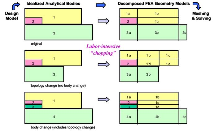
Figure 7. Variable Topology Multi-Body (VTMB) FEA Meshing Challenges
