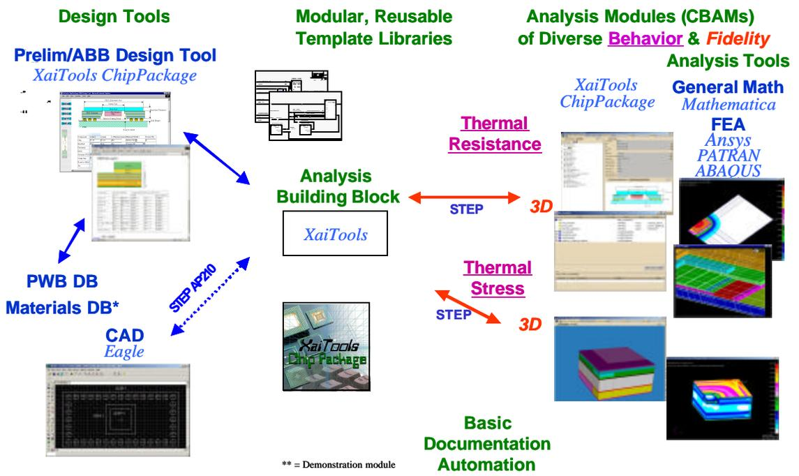
Figure 10. Flexible High Diversity Design-Analysis Integration
