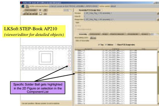
Figure 19. Chip package test case (in the STEP-Book AP210 tool after translation into the ISO 10303-210 neutral model format)
