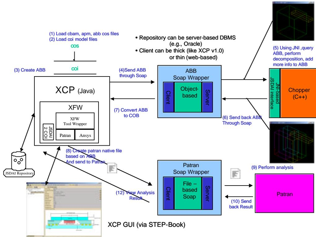
Figure 17. XCP Architecture (Developer's View)
