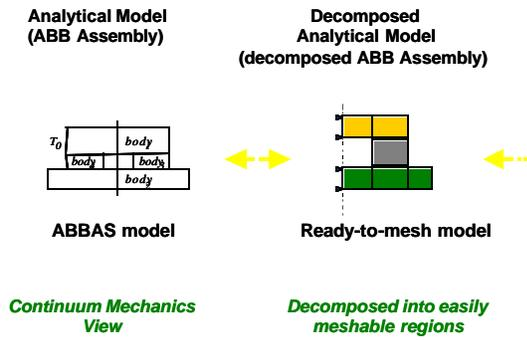
Figure 6. Main Stages at Level 3 for Generating Complex FEA Models
