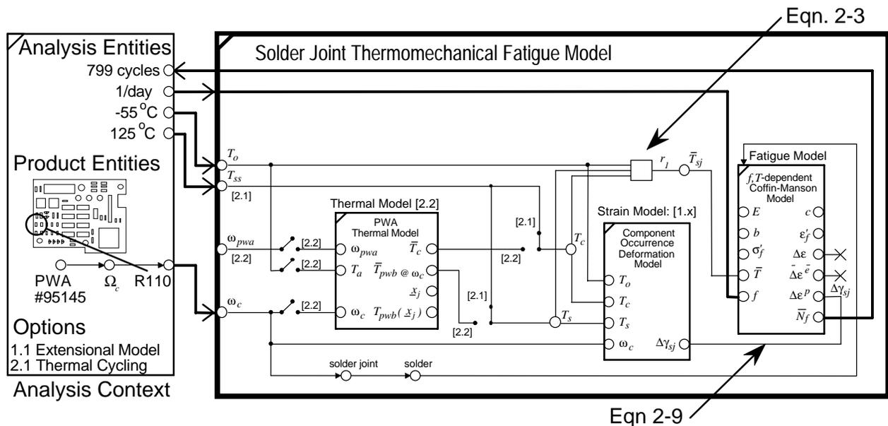
Figure 3-2 Solder Joint Thermomechanical Fatigue Model Instance View
