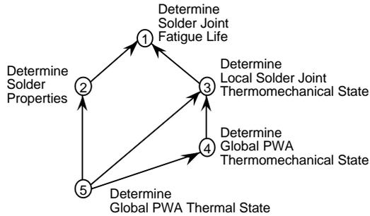
**Figure 2-1** Major Steps in Solder Joint Fatigue Analysis
