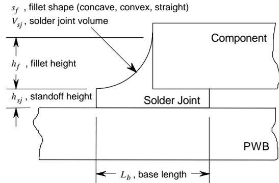
**Figure 2-4** Solder Joint Geometry
