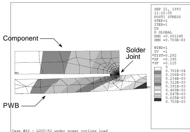
**Figure 3-6** Deformations with Rectangular Geometry Option
