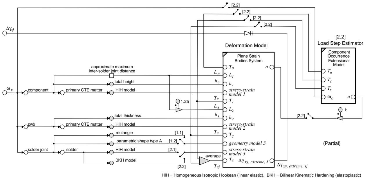
**Figure 3-4** Plane Strain Model Constraint Schematic
