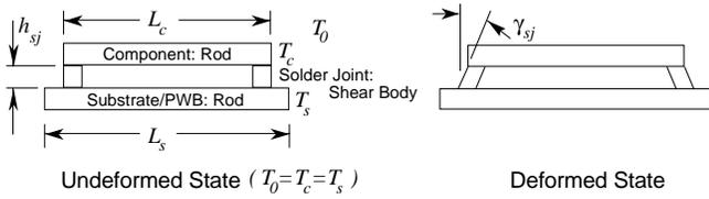
**Figure 2-3** Level 1 Extensional Model [after Engelmaier]
