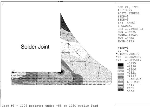
**Figure 3-7 Shear Stress in Detailed Solder Joint**
