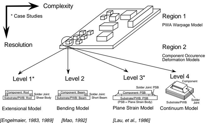
**Figure 2-2** Varying Levels of Thermomechanical Analysis Models
