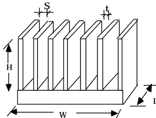
Figure 1. Prismatic Heat Sink
