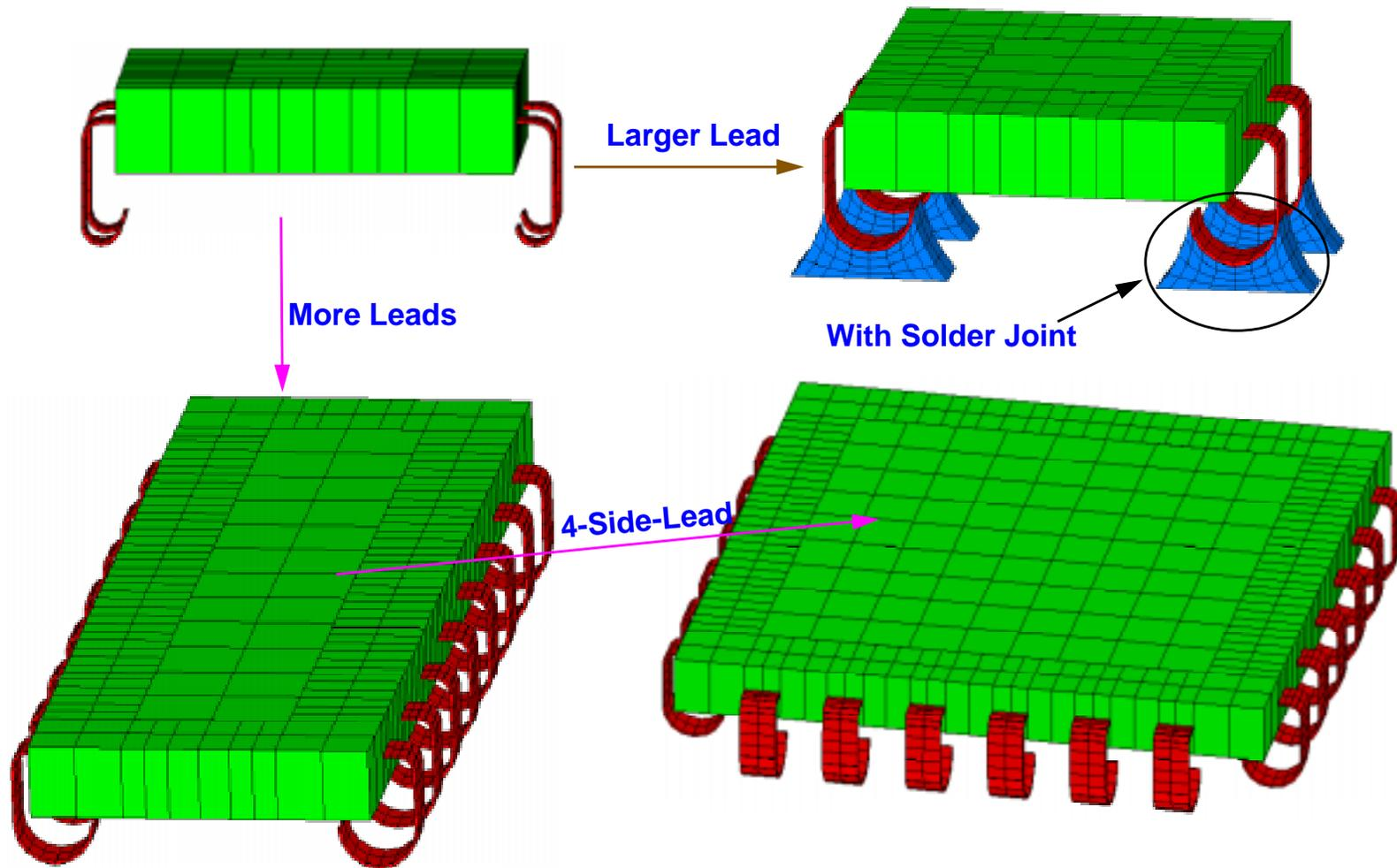
Figure 7.5 Parametric modeling for a TSOP component with J lead.
