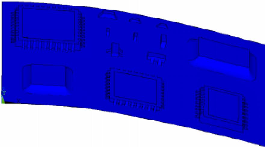
Figure 10.12 Deformed shape of a PWB under mechanical bending load.
