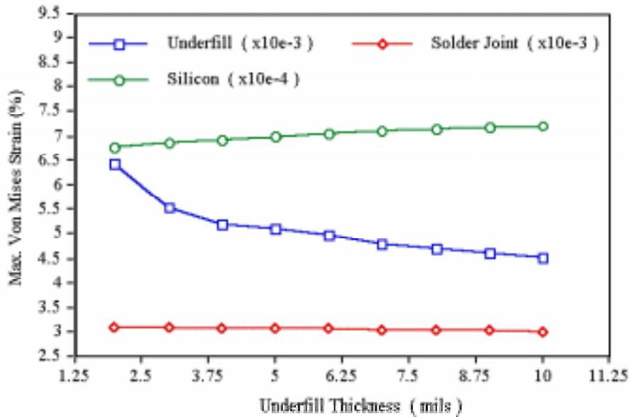
Figure 9.4 Parametric study results for underfill thickness.
