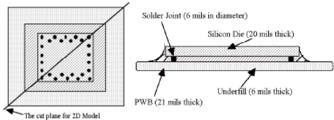
Figure 9.2: Schematic view of a typical FCOB structure
