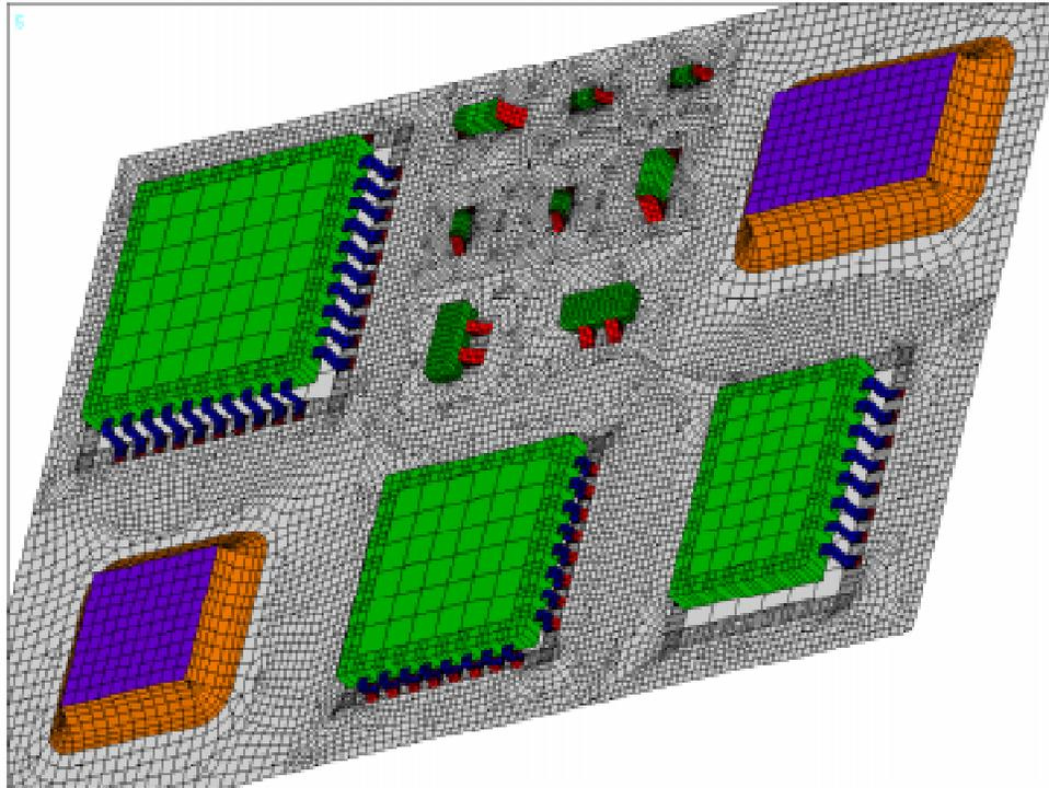
Figure 10.8 Re-mesh model after components rotation.
