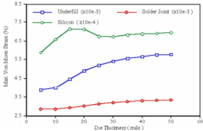
Figure 9.5 Parametric study results for die thickness
