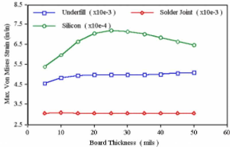
Figure 9.6 Parametric study results for board thickness.
