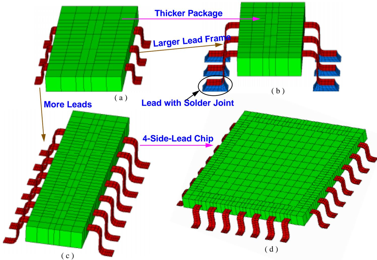
Figure 7.4 Parametric modeling of a TSOP component with gull lead
