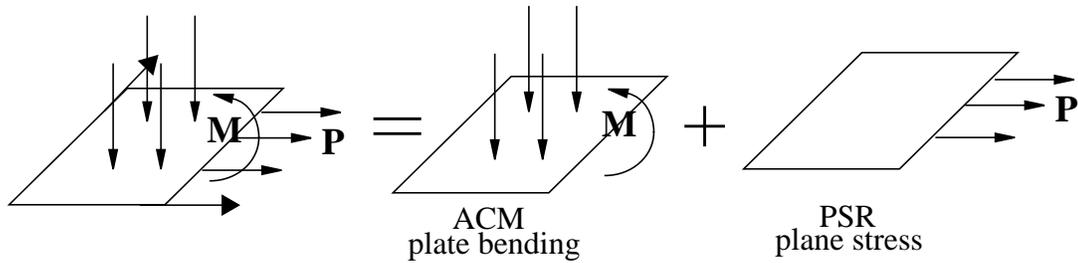
Figure 8.3 Selected stretching-bending shell element for PWB analysis.
