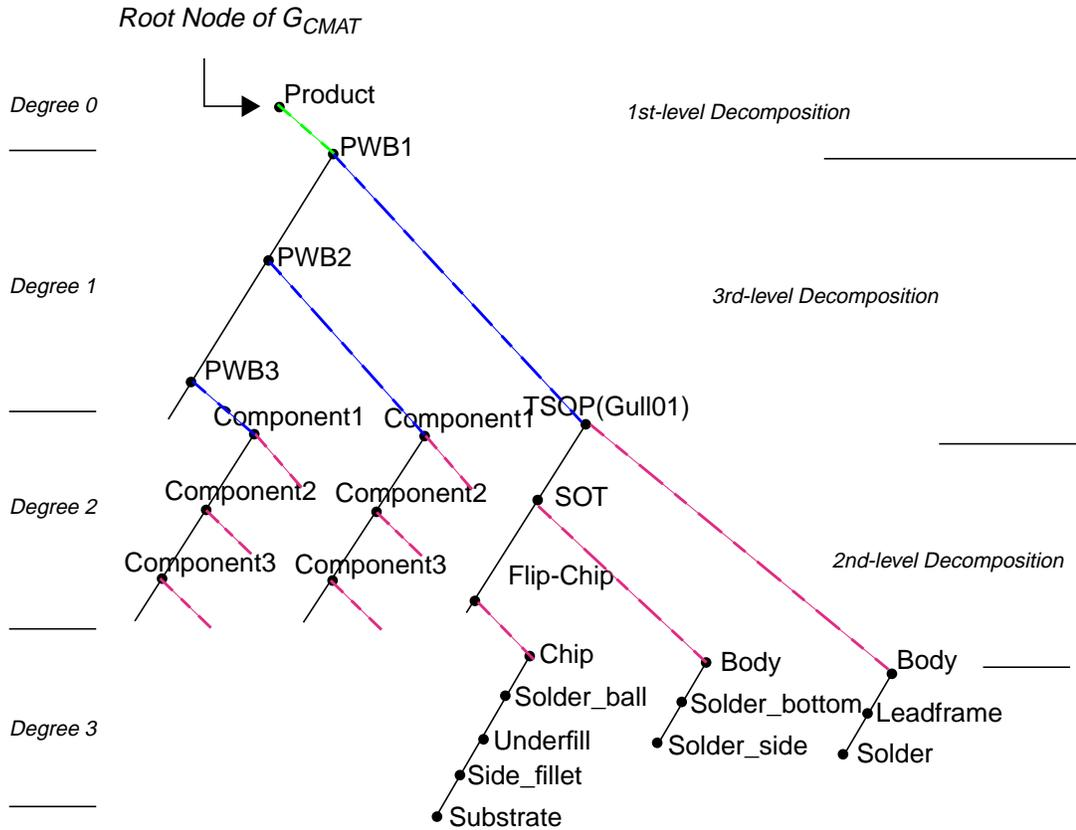
Figure 6.9 Graph representation of Constructive Module Assembly Tree (CMAT).
