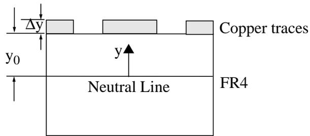
Figure 8.2 Cross section view of two layered board.
