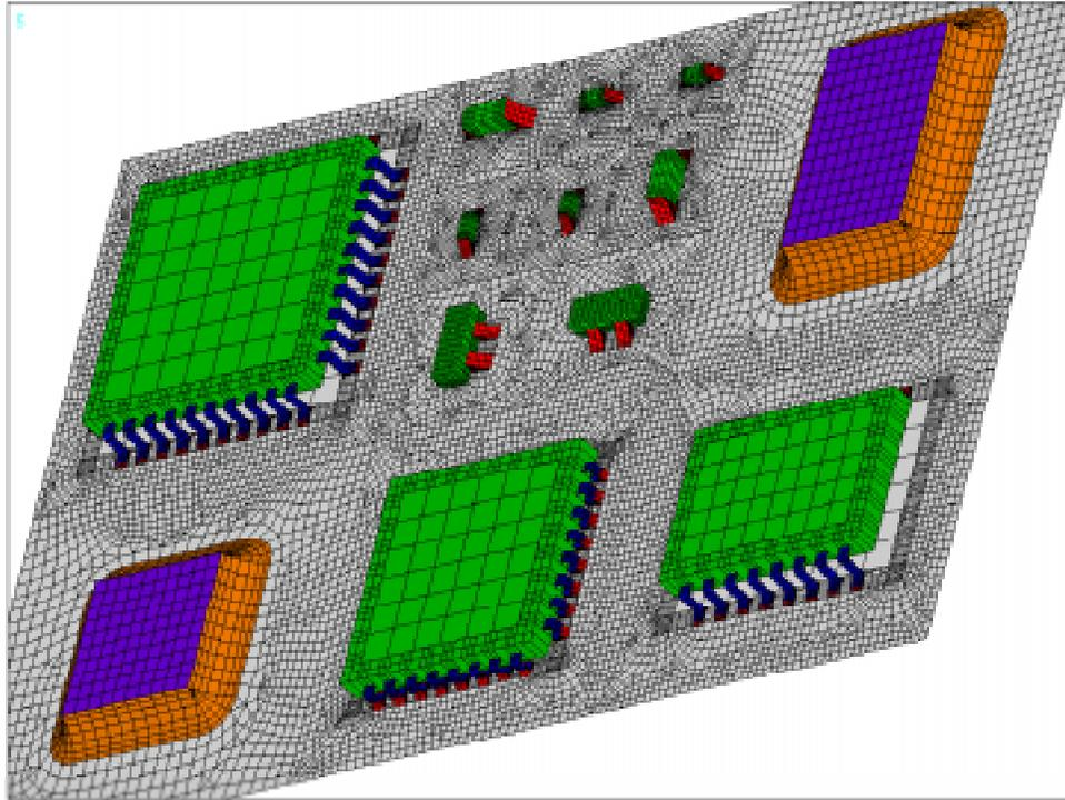
Figure 10.6 Completed FE model for the board and components.
