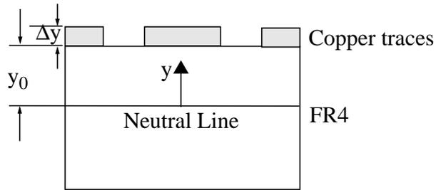
Figure 8.2 Cross section view of two layered board.
