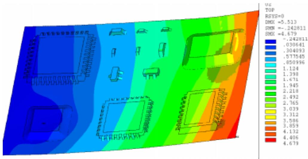
Figure 10.9 Warped board under thermal load.
