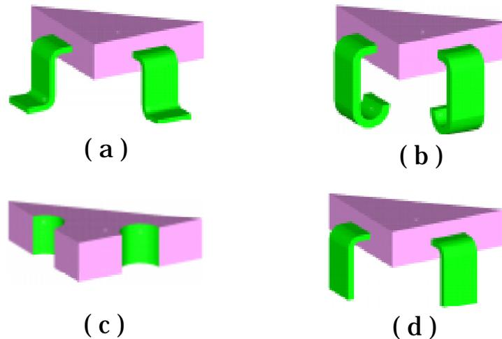
Figure 6.2 Taxonomy of active components. (a) Gull lead; (b) J lead; (c) Leadless; (d) I lead.
