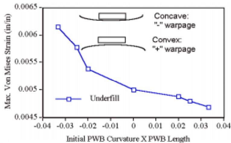
Figure 9.11 Parametric FEA results for initial warpage study
