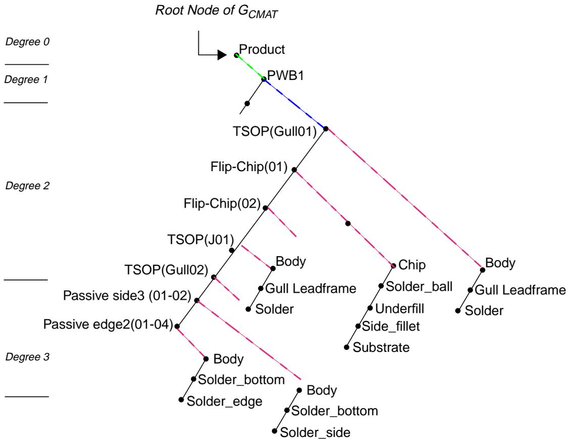
Figure 10.2 Construction of a CMAT for the PWB.
