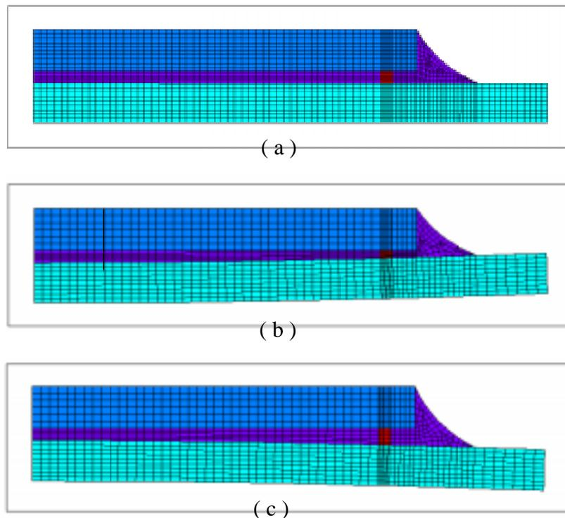
Figure 7.1 . Board initial condition: (a) flat; (b) warped-up; (c) warped-down.
