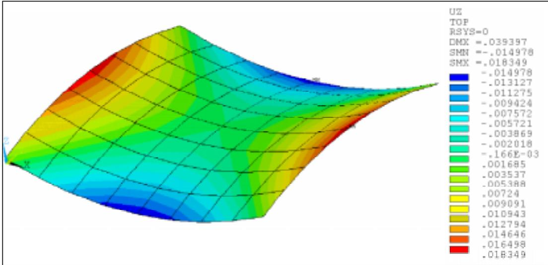
Figure 8.10 Warpage plot: Deformed PWB in a heating oven.
