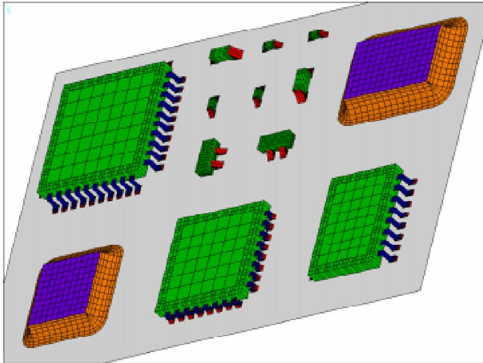
Figure 10.7 Modified FE model with rotated DCA and TSOP.
