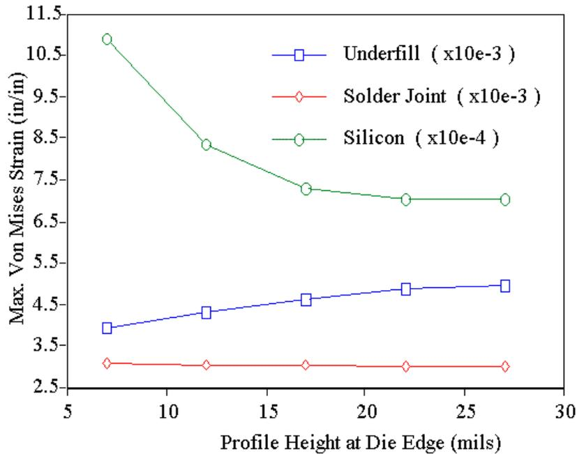
Figure 9.9 Parametric study results for underfill fillet height.
