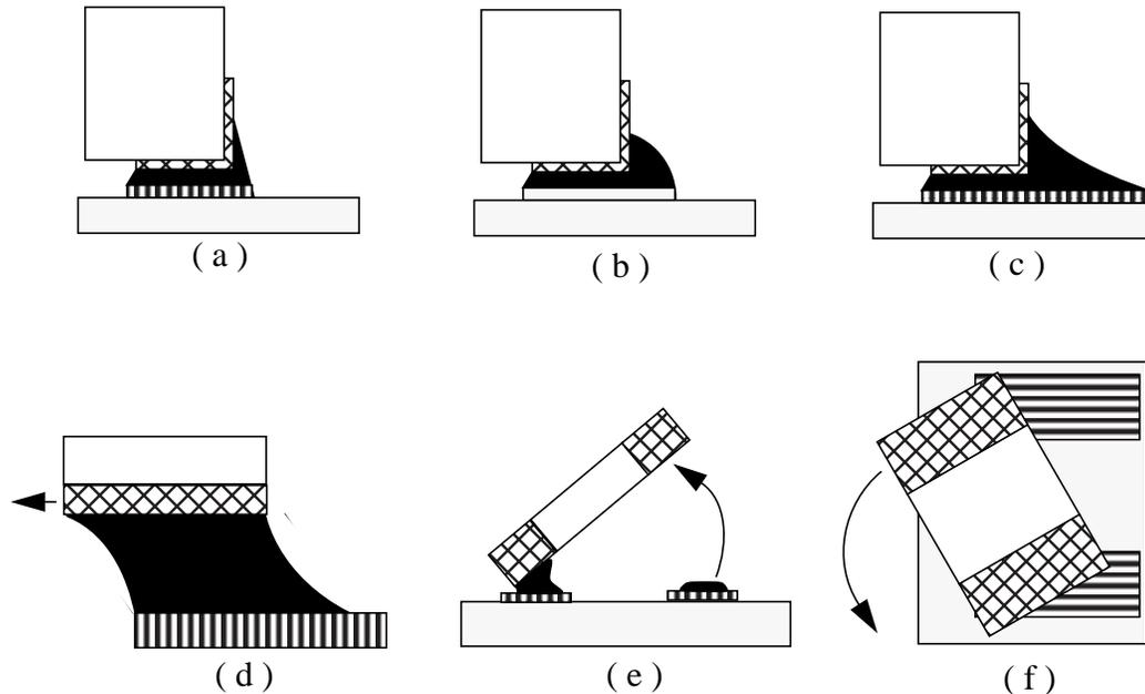
Figure 6.7 Taxonomy of solder joint variations: (a) insufficient solder; (b) optimal solder; (c) excessive solder; (d) mis-alignment; (e)tone-stone effect; (f) swimming.
