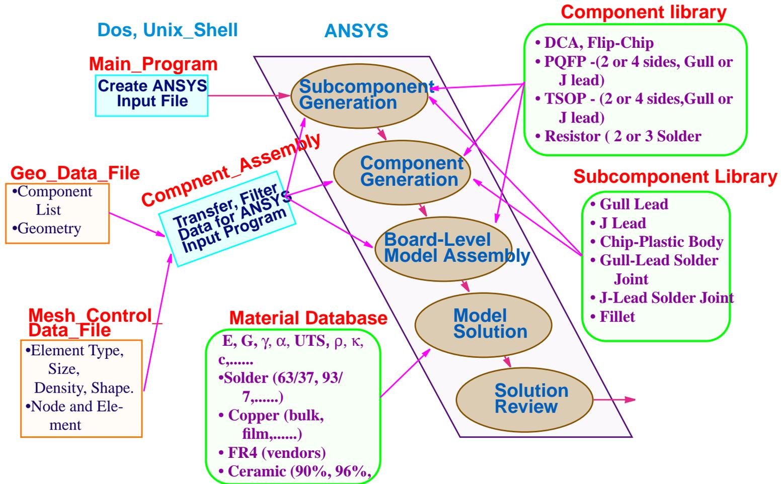
Figure 6.10 Program structure for a mechanical model assembly.
