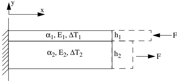
Figure 8.4 Two layered composite beam with thermal load.
