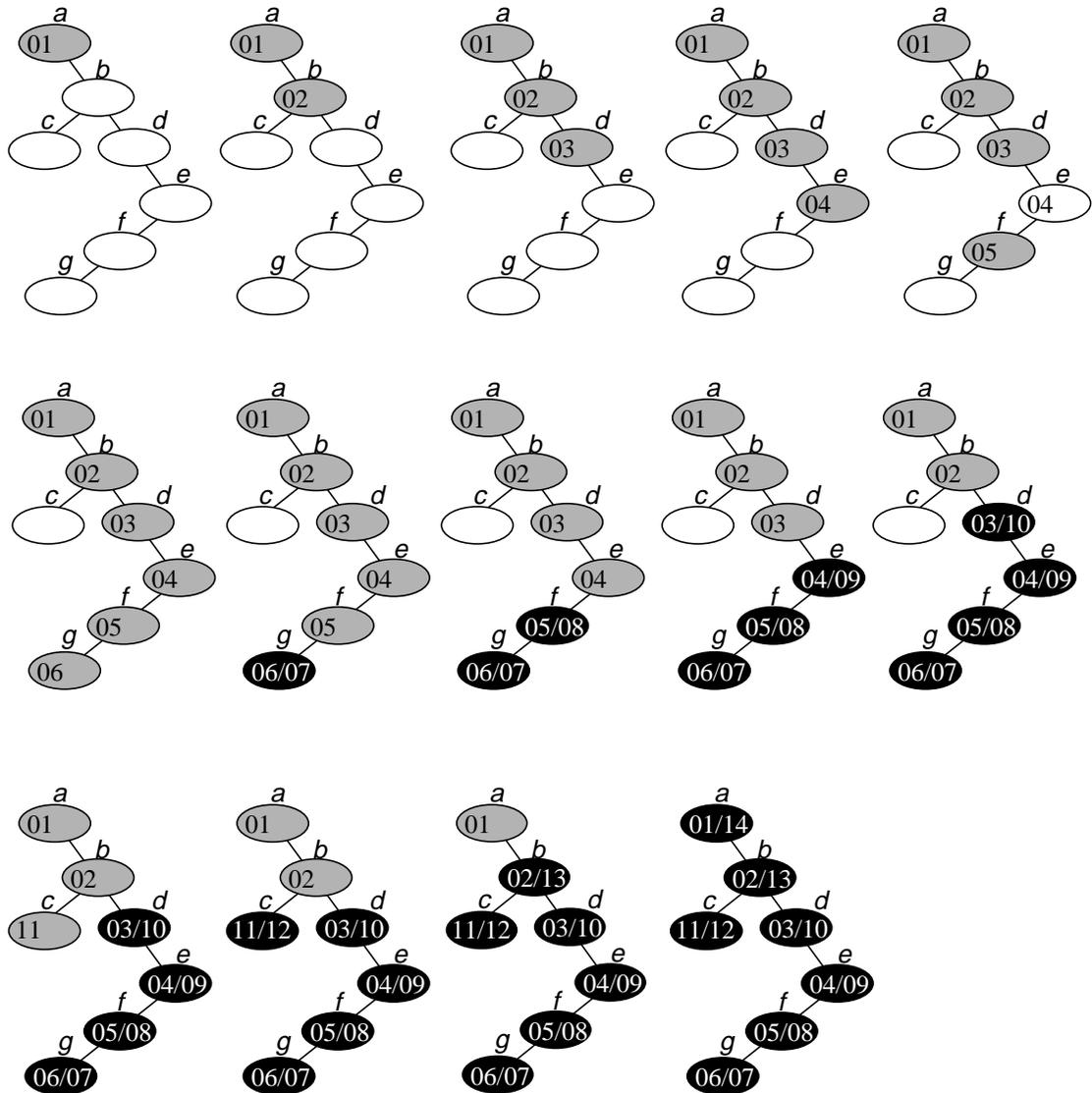
Figure 6.13 Exploration of a  $G_{CMAT}$  by DFS algorithm.
