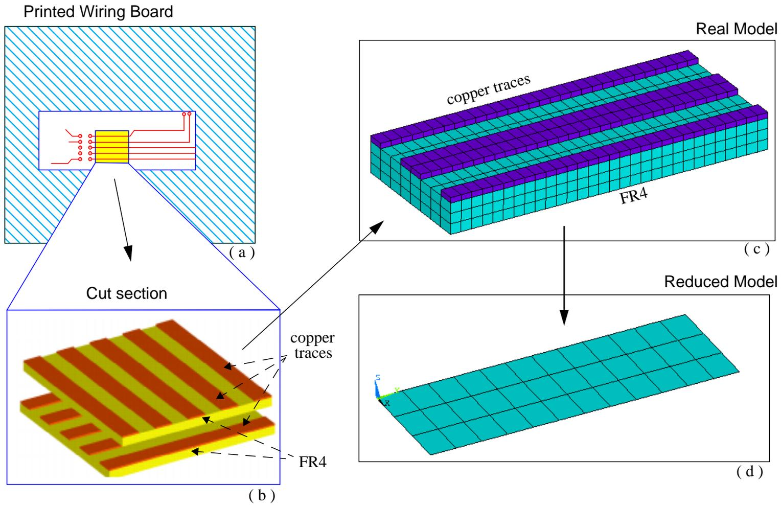
Figure 8.1 Divide-and-conquer algorithm for the modeling of a multilayer PWB.
