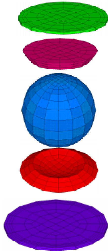
Figure 6.14 Modularized parts for a BGA modeling
