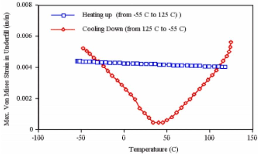
Figure 9.3 Maximum EEP in underfill (baseline configuration) during both cool-down and heat-up stage
