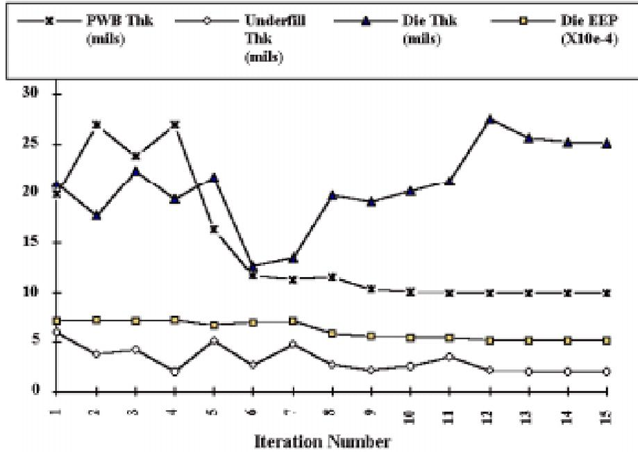
Figure 9.20 Design optimization for minimizing the die EEP
