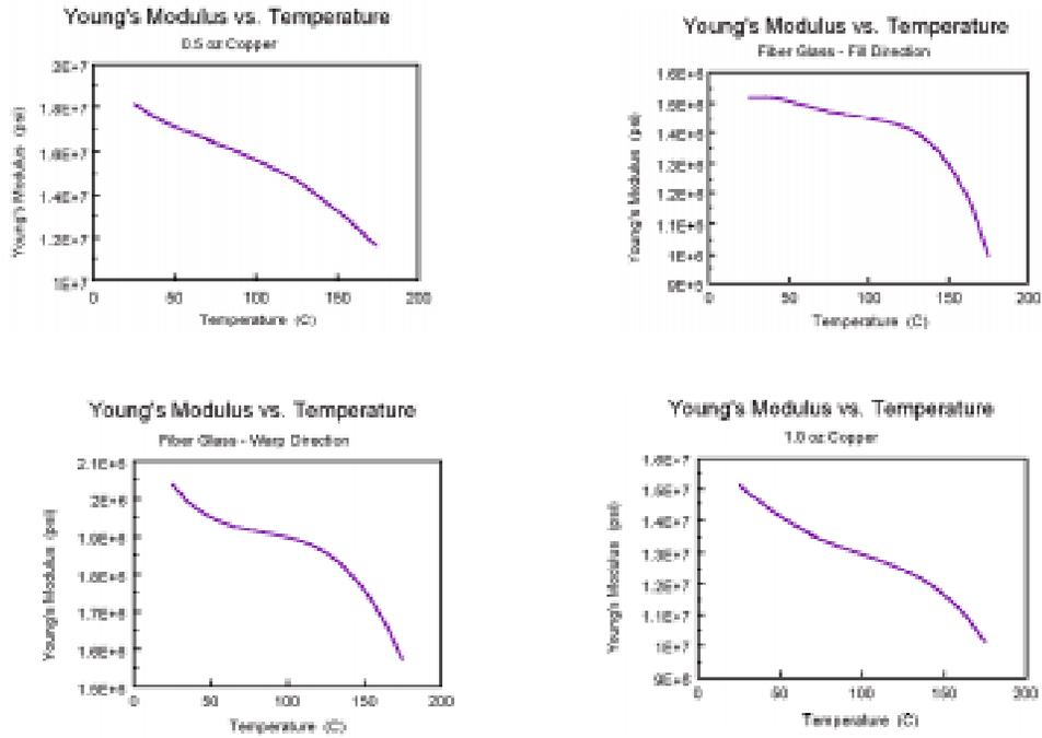
Figure 8.9 Material properties used for testing developed FE model.
