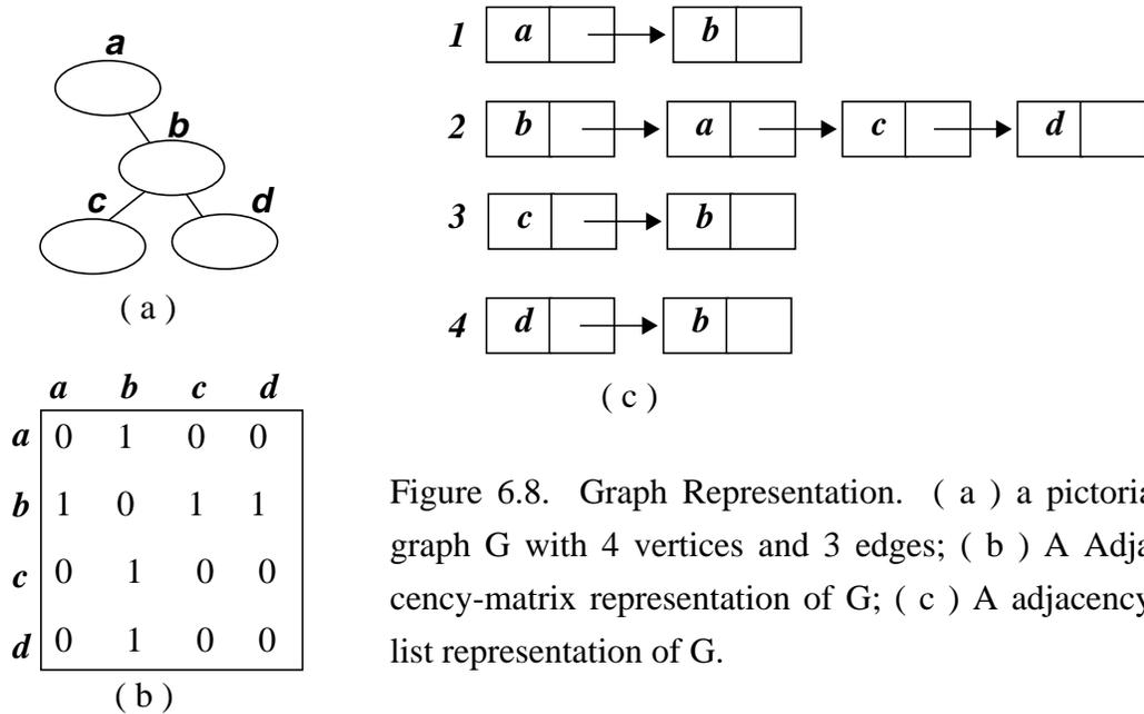
Figure 6.8. Graph Representation. ( a ) a pictorial graph  $G$  with 4 vertices and 3 edges; ( b ) A Adjacency-matrix representation of  $G$ ; ( c ) A adjacency-list representation of  $G$ .
