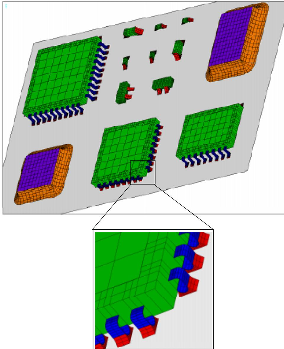
Figure 10.5 FE model for the components on the board.
