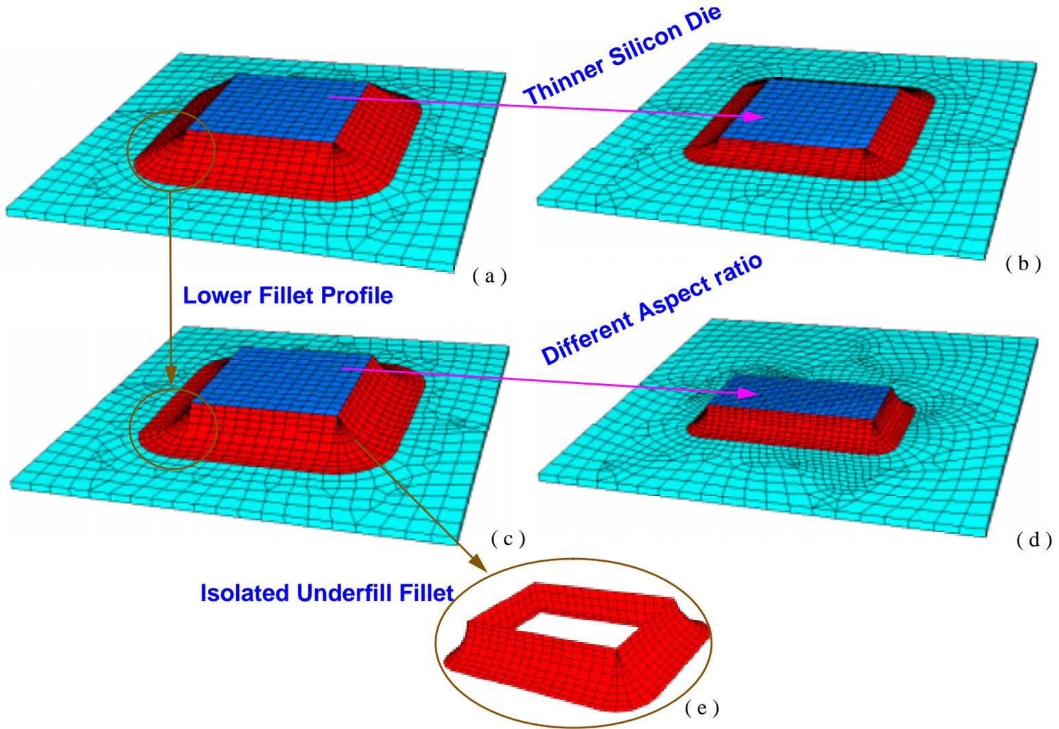
Figure 7.3 Parametric modeling of a DCA component.
