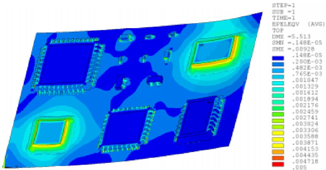
Figure 10.10 Strain distribution of the entire board under thermal load.
