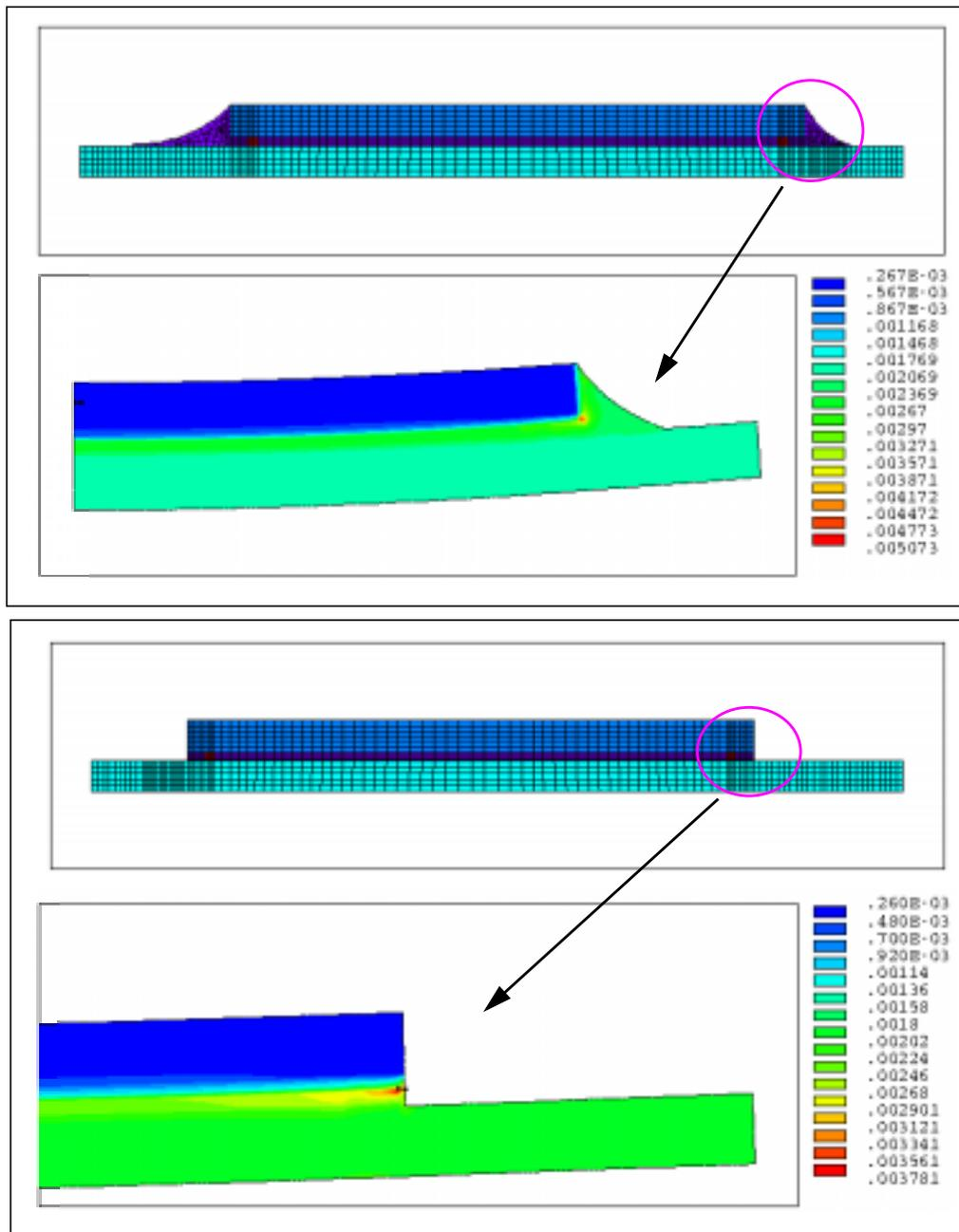
Figure 9.10 Parametric study for non-symmetric and no-fillet FCOB.
