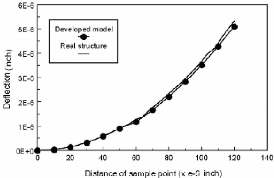
Figure 8.8 Comparison of a detailed FE model to a reduced model.
