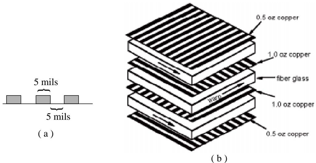
Figure 8.7(a) Cross section view of copper layer.
