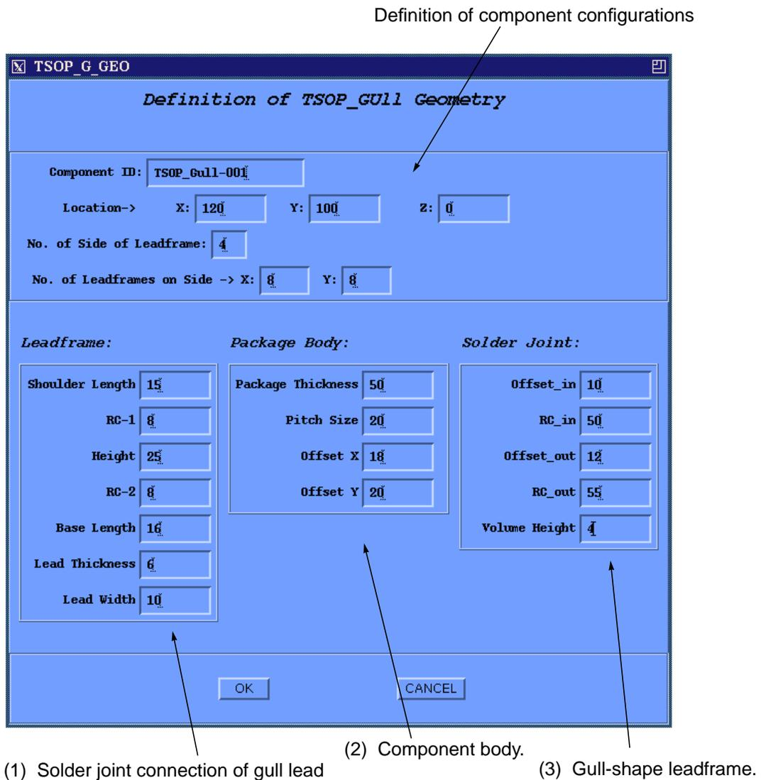
Figure 7.2 Definition of parameters for a TSOP component
