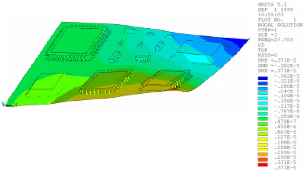
Figure 10.13 Deformed shape of a PWB under vibrational load (mode 3)
