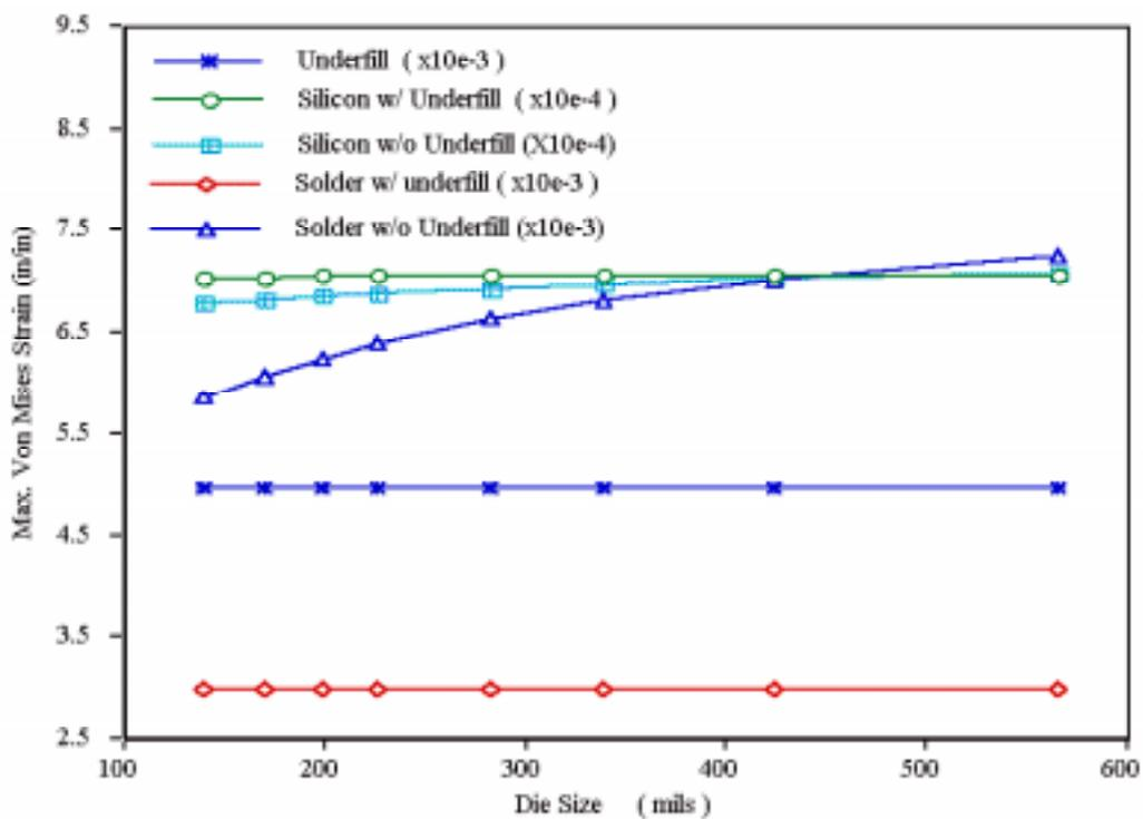
Figure 9.7 Parametric study results for die size
