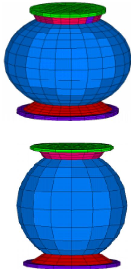
Figure 6.15 Two BGA FE models based on one modularized Model.
