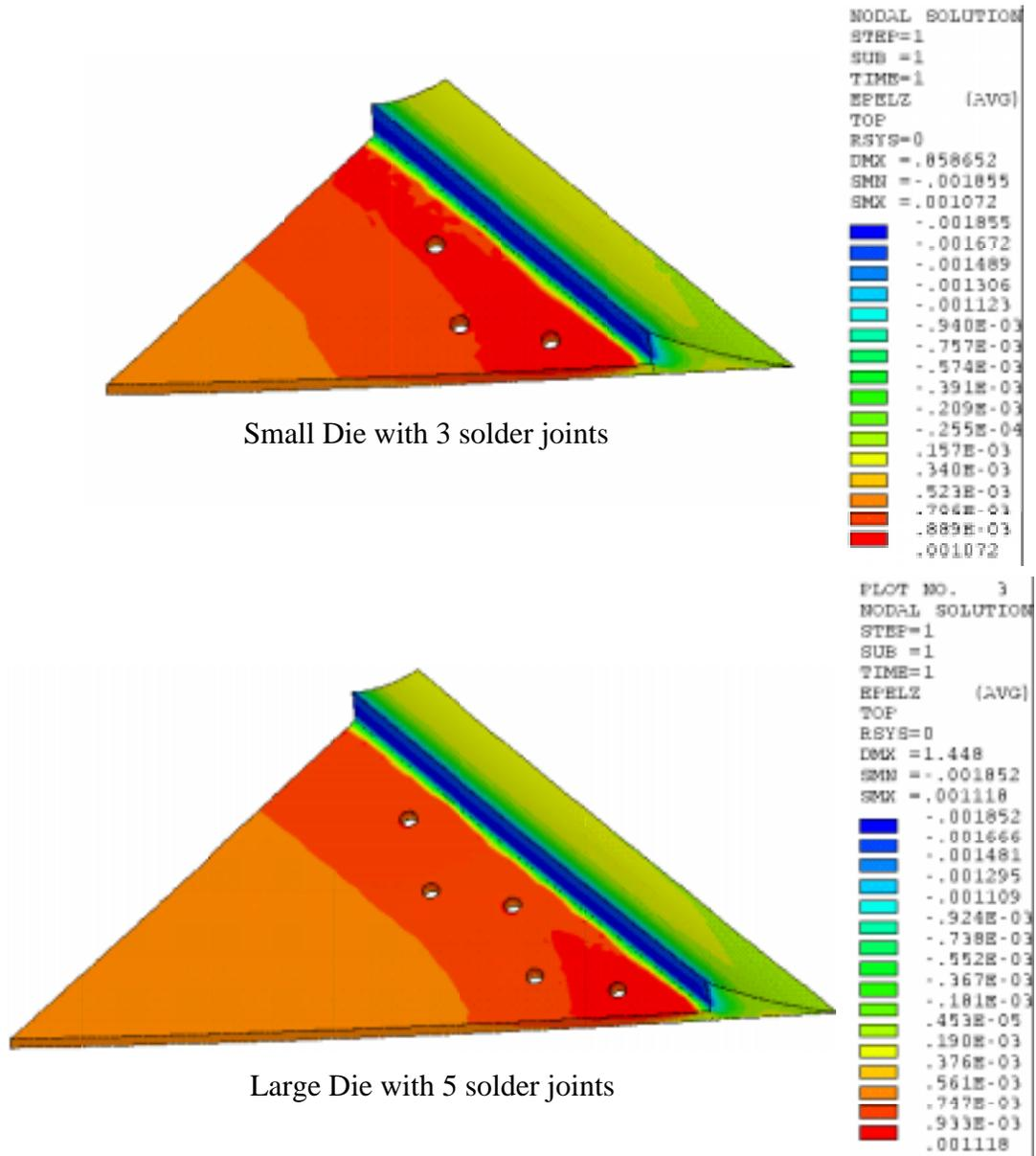
Figure 9.18 3D sensitivity studies of die size and solder location.
