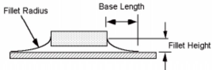
Figure 9.8 Key underfill fillet profile parameters.
